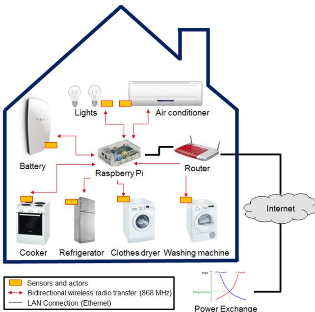
Fig. 1. Architecture of a smart home solution
